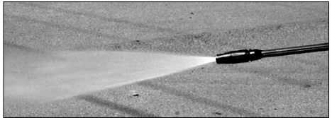
Figure 4 - Wide fan pattern
