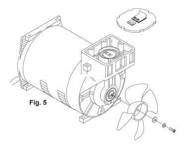
**STEP 10.** Install the fan onto the eccentric nib. Align the slot marked '8' with the notch on the eccentric nib. Tighten the screw and washer into the threaded hole in the nib. When properly assembled the fan will remain centered in the housing when rotated by hand.
